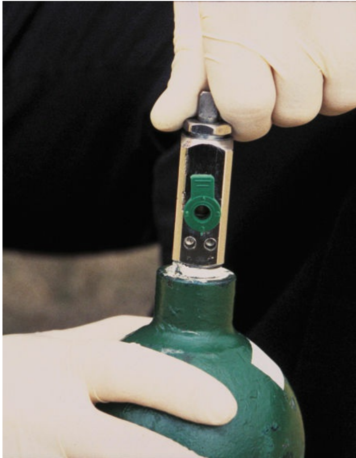
Figure 7-27 A valve stem with pin-index holes.
