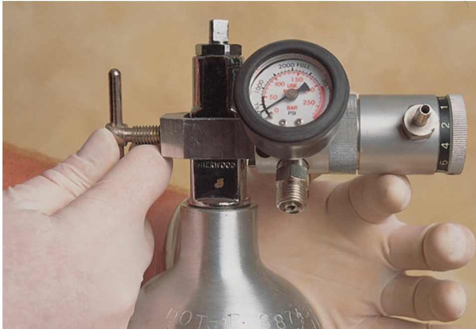
Figure 7-26 The regulator/flowmeter attaches to the outlet of the oxygen cylinder.
