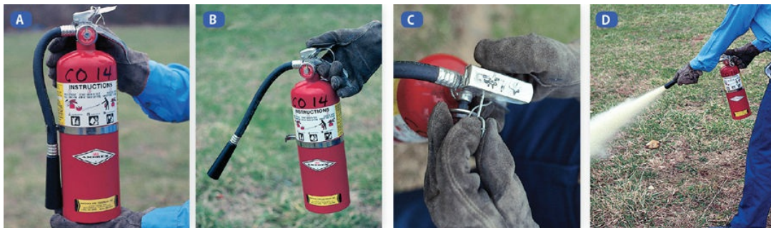
Figure 20-6 Use of a dry chemical fire extinguisher. A. Check the pressure gauge. B. Release the hose. C. Pull the locking pin. D. Discharge at the base of the fire.
