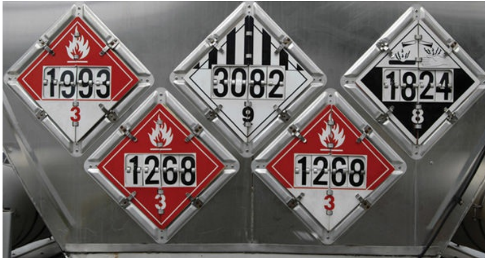
Figure 11-7 Placards used to identify the presence of hazardous materials.
