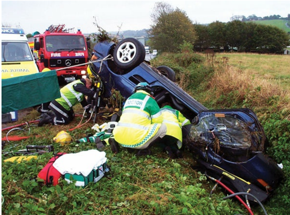
Figure 20-3 A vehicle positioned on its side is obviously unstable.
