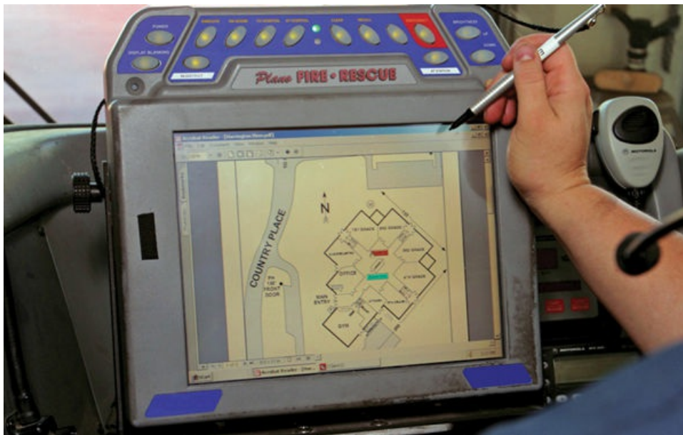
Figure 5-2 A mobile data terminal (MDT) can be used to display routing information transmitted from the dispatch center.
